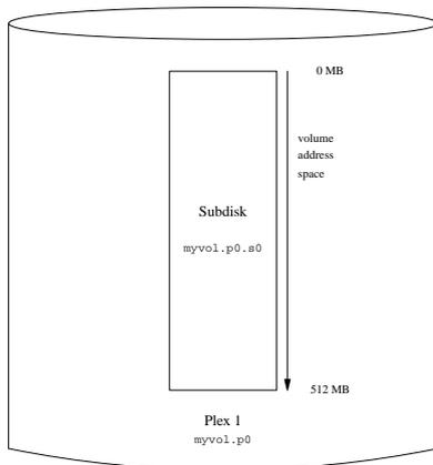
This figure, and the ones which follow, represent a volume, which contains the plexes, which in turn contain the subdisks. In this trivial example, the volume contains one plex, and the plex contains one subdisk.
