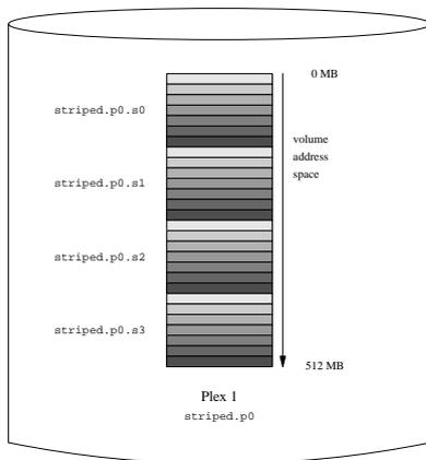
This volume is represented in 圖形20-6. The darkness of the stripes indicates the position within the plex address space: the lightest stripes come first, the darkest last.
