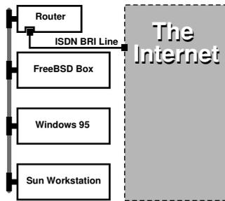
If your home/branch office is only one computer you can use a twisted pair crossover cable to connect to the stand-alone router directly.
