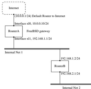
In this scenario, RouterA is our FreeBSD machine that is acting as a router to the rest of the Internet. It has a default route set to 10.0.0.1 which allows it to connect with the outside world. We will assume that RouterB is already configured properly and knows how to get wherever it needs to go. (This is simple in this picture. Just add a default route on RouterB using 192.168.1.1 as the gateway.)
