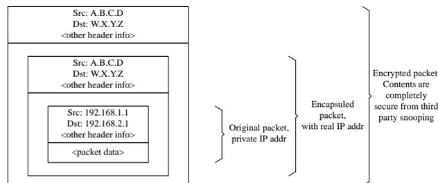
When they are received by the far end of the VPN they will first be decrypted (using the security associations that have been negotiated by `racoon`). Then they will enter the `gif` interface, which will unwrap the second layer, until you are left with the innermost packet, which can then travel in to the inner network.
