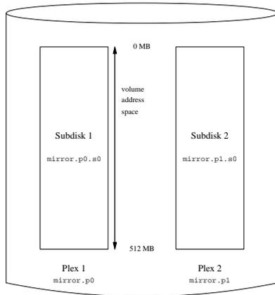
In this example, each plex contains the full 512 MB of address space. As in the previous example, each plex contains only a single subdisk.
