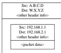
This encapsulation is carried out by the `gif` device. As you can see, the packet now has real IP addresses on the outside, and our original packet has been wrapped up as data inside the packet that will be put out on the Internet.
