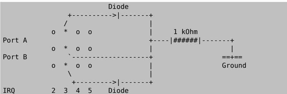
The cathodes of the diodes are connected to a common point, together with a 1 kOhm pull-down resistor. It is essential to connect the resistor to ground to avoid floating of the IRQ line on the bus.
