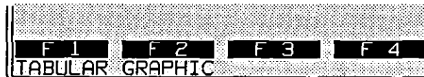
Figure 6-25 The two types of statistics display are accessible in Run mode on the second rack of softkeys.
