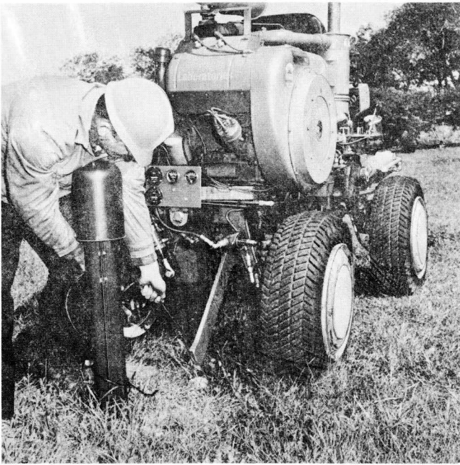
Fig. 15-26 — Vibrating Lawn Plow
