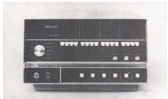
Fig. 2 IMP-16L. National Semiconductor Corp offers this prototyping system for use with its IMP-16 microprocessor. Control panel is both an operator's console and a programmer's panel
