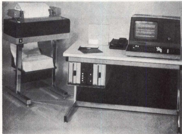
Basic DMS microcomputer system containing dual-drive DynaTerm-Disk ® , 8K RAM, software, and two RS-232-C ports for terminal and line printer interfacing is a hardware/software tool for developing custom software for 6800 systems
