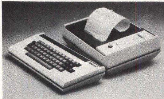
Telpar's PS-48C interactive thermal printer also serves as full-duplex, bit serial I/O terminal with addition of optional keyboard
