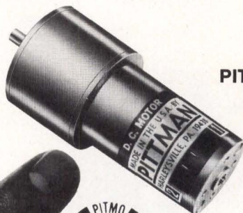
LO-COG® Servo Motors 3 series: 1.2, 1.6 and 2.0" OD Stall torques: about 1 to 128 oz.-in.
