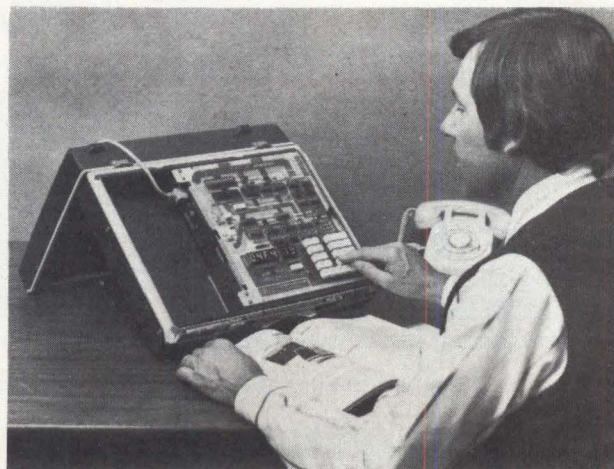
Microprocessor lab from Hewlett-Packard trains user in areas of troubleshooting, hardware, and software. Block diagram layout of main circuit board uses color graphics to teach hardware concepts; Monitor program demonstrates programming aspects; and addition of signature analyzer supplements troubleshooting experiments
