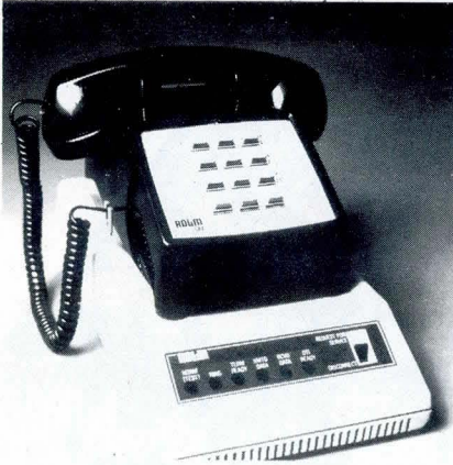
Fig 1 Data terminal interface module. Front panel toggle switch originates call, disconnects call in progress, or manually answers incoming call. Six LEDs indicate power and DTI and data signal status. Switch mounted at rear of unit is used for testing and for switching to automatic answer mode
