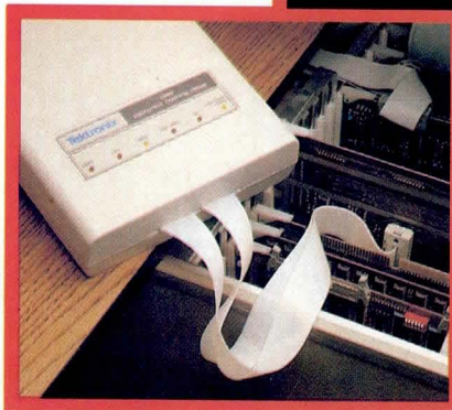
6809 Prototype Control Probe tip fits easily in hard to reach locations. Probe status lights monitor key processor signals.
