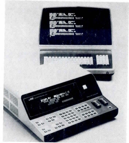
Microsystem emulator enhancements. Offered by Millennium Systems, Inc, interactive CRT terminal display capability and additional 8k bytes of RAM increase versatility of Microsystem Emulator
