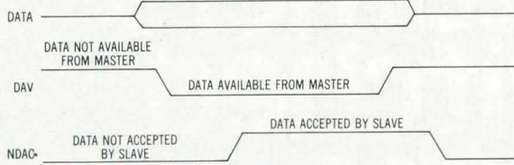
Fig 2 Timing diagrams for double-buffered conditional output with two flags. With two flags, there must be four different logic states: two for DAV flag and two for NDAC flag
