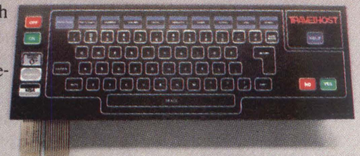
The videotex terminal for the hotel/motel room, designed and manufactured by Dallas based QUAZON CORPORATION for the Travelhost Network, features this MICRO SWITCH custom touch panel.
