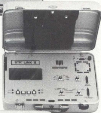
8-bit parallel STR-110 allows memory dumps or program loading up to 125 characters per second. $1328 in single quantity.
