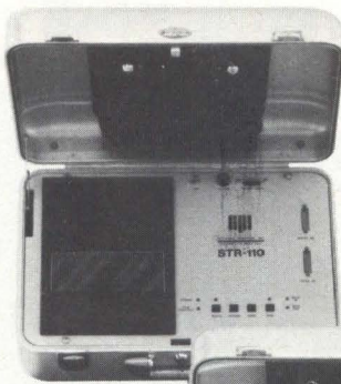
8-bit parallel STR-110 allows memory dumps or program loading up to 125 characters per second. $1328 in single quantity.
