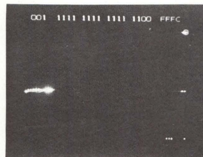
Fig 3 Map display for valid program execution. Analyzer triggers on start location FFFC. Cursor (boxed point) is placed at trigger and displayed at top of screen. 507 memory accesses after trigger are mapped
