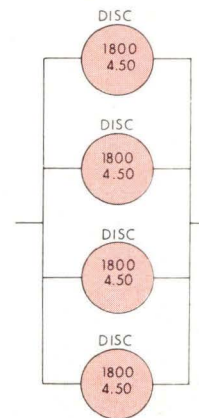
Fig 4 Paralleling elements increases reliability. Parallel subsystem works as long as any one of its constituent elements operates. This computer system is usually energized by one of its redundant uninterruptible power supplies. Should both these power sources fail, bypass transfer switch connects ac bus to normal utility company voltage
