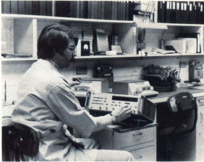
Fig 3 BER test setup. Test instrument HP1645A has been set to proper clock frequency and has completed proper handshake signals to accomplish transmission
