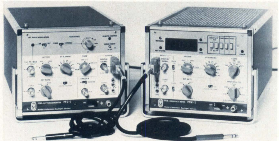
PF-1C test setup. It has compatible 100/110- \Omega balanced inputs and outputs and provides standard T1 (AMI-1/2) and T2 (B6ZS) line codes. There are additional 75- \Omega inputs and outputs with RZ, NRZ, and AMI-1 codes
