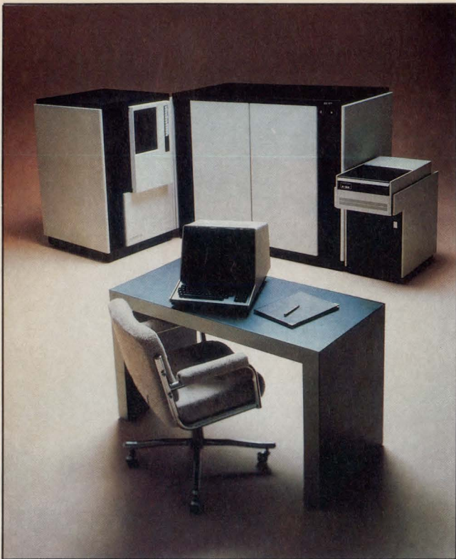
CPU, IPU, and floating point processors in Gould's Concept 32/87 minicomputers are implemented in 10K ECL. The systems attain 4 MIPS performance levels through large cache memory, 4-stage instruction pipeline, and dual instruction/execution unit architecture.
