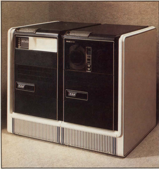
The MV/4000, Data General's low end 32-bit ECLIPSE, rated at 500K Whetstones/s, supports 8M bytes of main memory and accommodates 64 terminals. Housed in a 1-m high cabinet, the system's 2-board CPU takes advantage of gate array and programmable array logic technologies.
