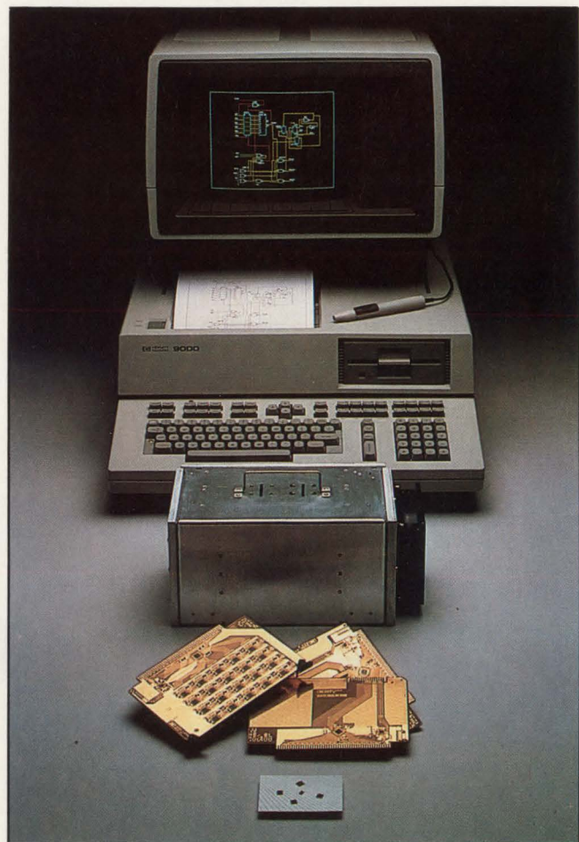
Based on a VLSI 5-chip set, the processor in the HP 9000 packs in key functions of a 32-bit mainframe computer. Slightly larger than a personal computer, the desktop workstation uses a multiple processor architecture to offer three levels of performance by plugging in up to three CPU boards.
