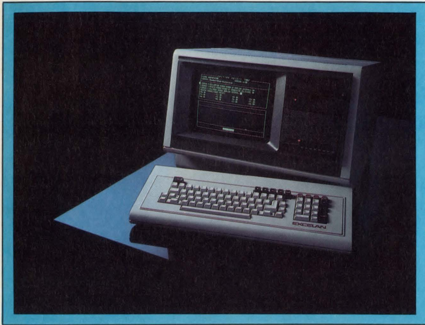
Excelan's Nutcracker is a standalone workstation for controlling and monitoring Ethernets. With its combination of high speed TTL hardware and object-oriented software a net manager can monitor and control traffic, as well as identify problems.
