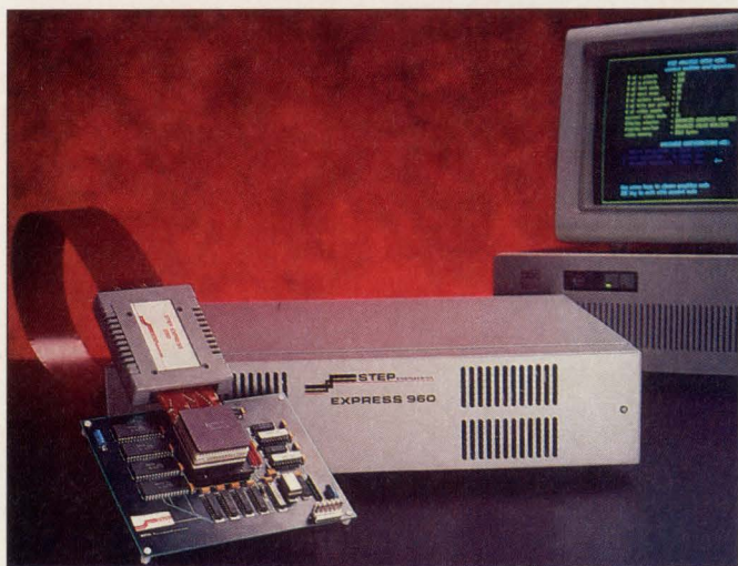
Real-time development tools for RISC processors are rapidly becoming available. The Express Plus by Step Engineering is an emulator for the Intel i960CA superscalar processor which can run at up to 33MHz. The emulators are available with a selection of integrated compilers, debuggers and other development software.
