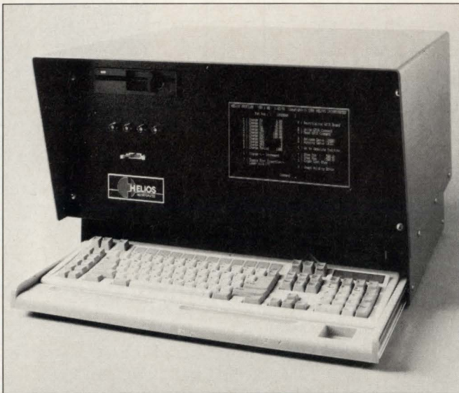
The Proteus system simulates a disk-drive's servo signal and mechanical HDA characteristics before the drive is built.
