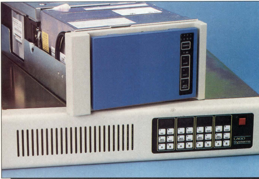
Our Lago box allows us to use drives, such as the Imprimis (CDC) Sabre, as MSCP-served disks on our cluster.
