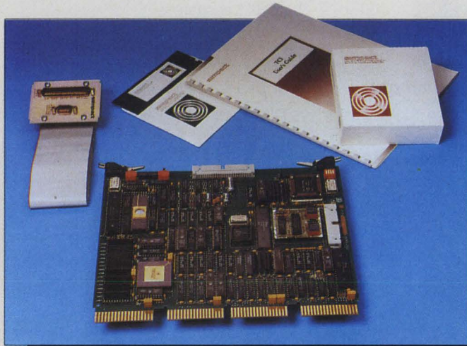
Simpact Associates Inc.'s TCI 2000 Series lets a MicroVAX connected to a Token Ring look like a Token Ring node.
