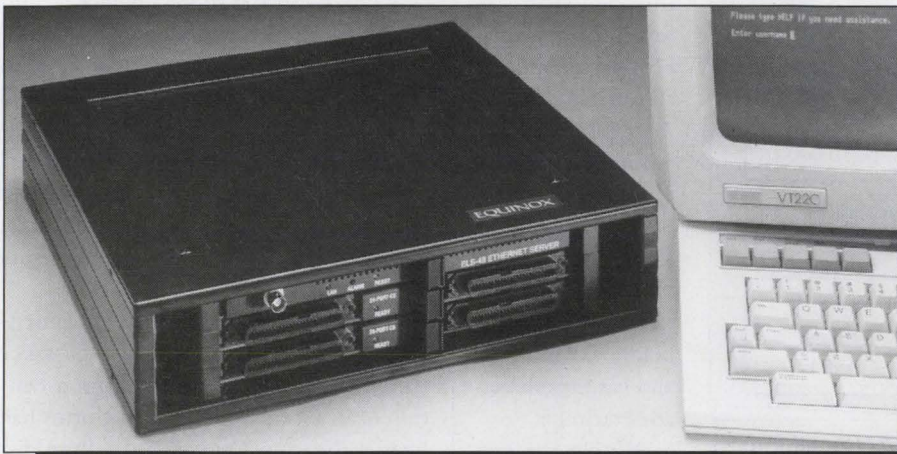
Equinox Systems Inc.'s ELS-48 terminal server uses DEC's LAT protocol.
