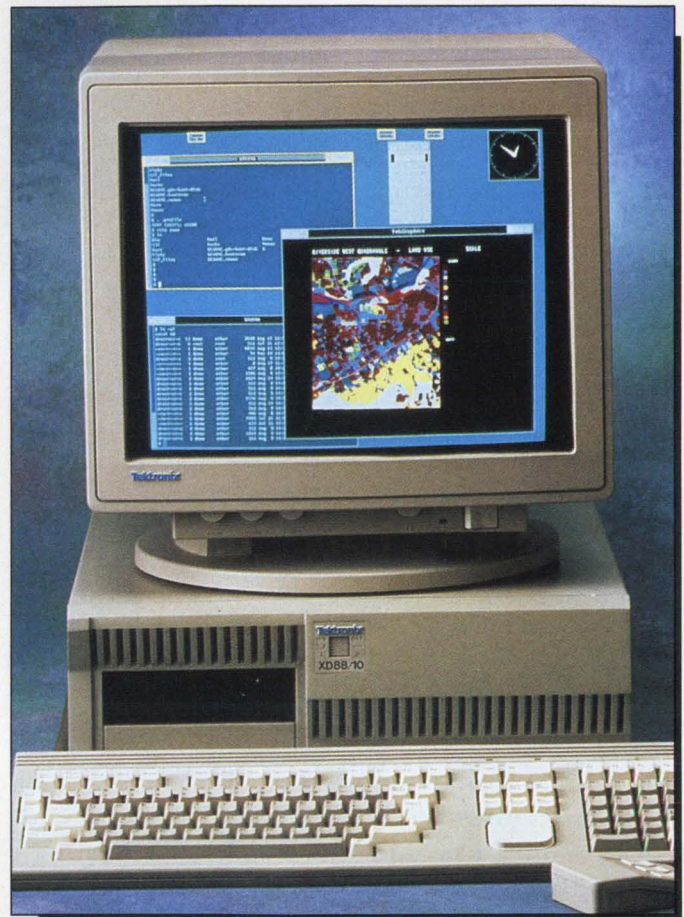
Tektronix Inc.'s XD88/10 graphics superworkstation is based on the Motorola 68020 graphics engine and 88000 RISC chip.
