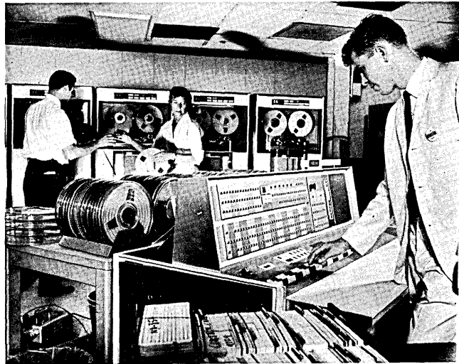
A duplicated mag tape is mounted on one of NAA's six 7090s following microwave transmission from Oat Mountain.
