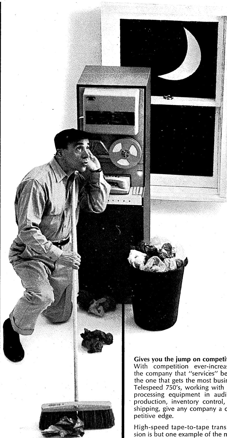
The Telespeed 750 receiving set collects all branch office data recorded on the punched tape; all automatically, all unattended.
