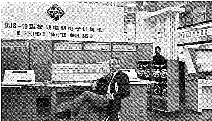
The author is shown at the console of the DJS-18 in Canton. A third generation machine, it's rated at 150,000 operations/sec, and supports a 65K (48 bit words) 2-usec core memory. Just to his right are paper tape drives and the plotter.
