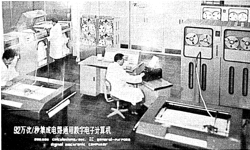
The peripherals on this 920K operations/sec IC machine all differ from those shown in other photographs. This installation is thought to be in Shanghai.
