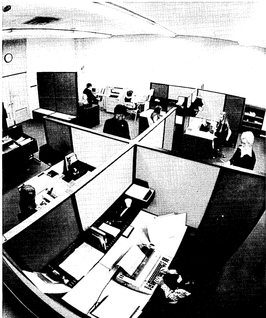
THIS WORD PROCESSING center at the main office of First Federal Savings and Loan Assn. of Broward County, Ft. Lauderdale, Fla., is one of three for the association. Each uses an IBM 6/450 information processor (left rear) combined with mag card typewriters and 6:5 cartridge systems and IBM dictation equipment.
