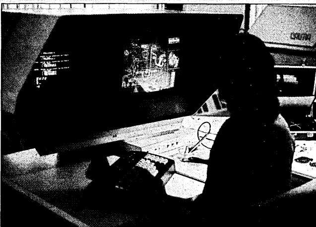
THE CALMA DUAL-CRT WORKSTATION allows GE employees to view both the circuit breaker design and its specs at the same time.
