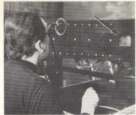
Experimental subject attempts to match movement of two light spots on a 5" CRT (arrow) while also responding to secondary stimuli from lamps and LEDs ringing the CRT. Sensor in ring tracks eye movement.
