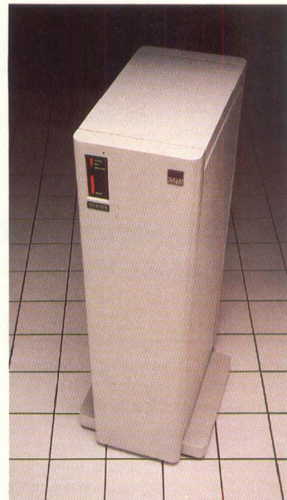
Figure 3: The Mach 1000, a logic simulation accelerator from Silicon Solutions, is built around the CADAT simulation algorithm and includes 10 full custom ICs, a 68010 front-end processor and up to 8 Mbytes of main memory. Special emphasis has been put on developing a compiler that speeds both design flattening and interconnection, and provides incremental compilation.
