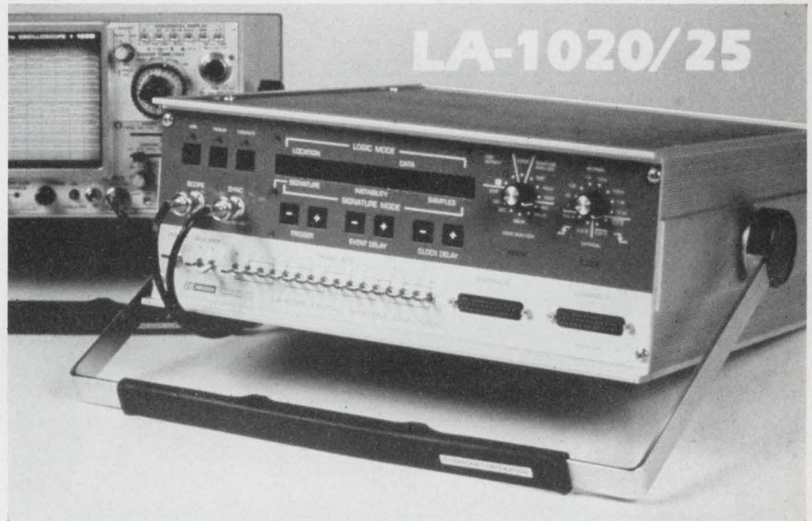
Figure 1: Dolch has placed a huge demand on their logic analyzer's operational parameters. They have recognized ICE (In-Circuit-Emulation) as an extremely powerful analytical methodology to follow in software testing. By creating an interaction in ICE, they have gained control of program execution, thus allowing the read-out of initial CPU register values, which cannot be seen directly through the monitoring bus. Equally as important, word-generation is possible.
