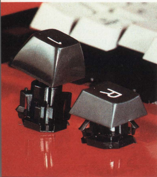
Figure 5: Keys of Micro Switch's low profile keyboard show reduced height.
