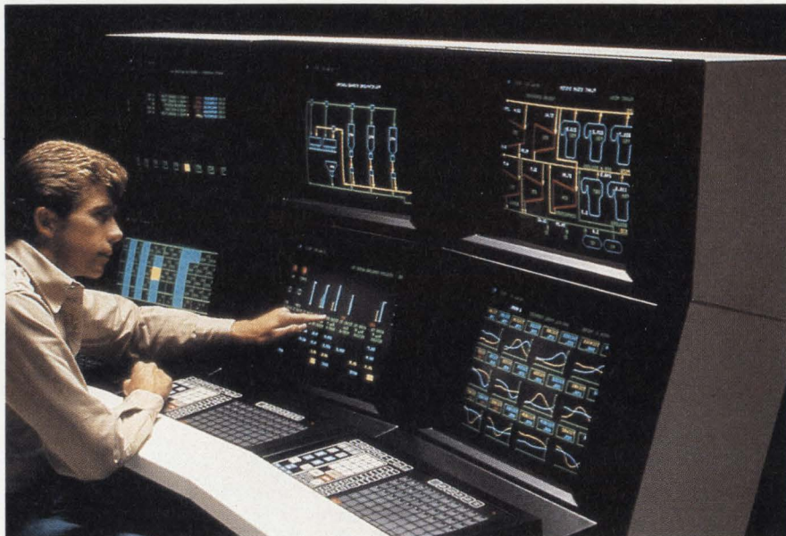
Honeywell TDC 3000 process management system fully integrates process control and plant information.
