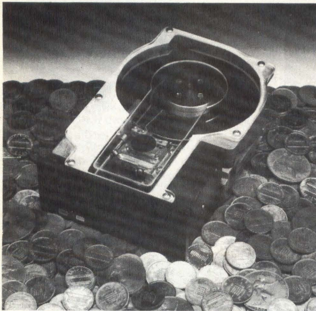
Figure 4: Newbury Data's four-platter Penny Winchester is the first 50-Mbyte 3½" Winchester.
