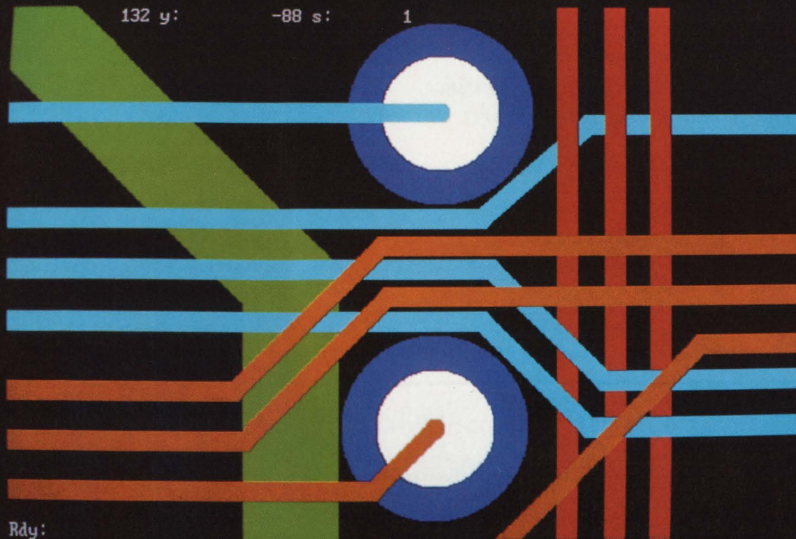
Pictured above is a DRAFTSMAN-EE™ screen of a four-layer board routed by DC/AUTOROUTER II™. The blue circles represent outer layer pads while the white circles represent inner layer pads. The one-mil diagonal DC/AUTOROUTER II™ makes the most of any routing situation putting as many traces between pads as your design rules allow. The professional straight-line routing is a result of the final via minimization and route-straightening pass.
