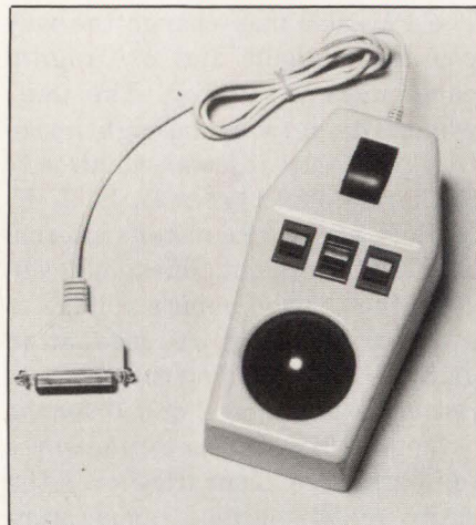
Providing 3-dimensional cursor control at a resolution of 200 pulses/in., the FastTrap pointing device plugs into the serial port of any IBM PC or compatible computer via its RS-232C interface.
