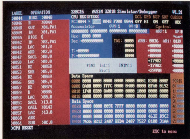
Fig 6 —The screen of the Avsim simulator may look confusing, but in fact it's very easy to use. We used the simulator to debug the transponder code. Here, the simulator is waiting for BIO to go low before it will accept a sample. The cursor is on the BIO pin. To allow the program to proceed, all we need to do is enter a 0 and watch the program accept the sample.
