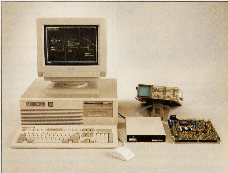
Combining the Sproc 1400's multiprocessing architecture with the company's development tools allows you to design analog and digital signal-processing functions at the block-diagram level. Without your having to write any code, software then automatically allocates execution tasks to each processor for the fastest runtime.
