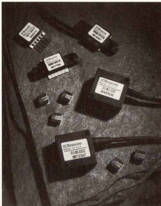
Accelerometers come in a variety of packaging options, from surface-mount sensor-only devices to encapsulated sensors with built-in signal conditioning.
