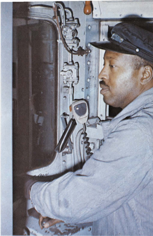
The speaker mike at the right of this motorman connects to a transceiver that plugs into a dc outlet aboard the train. The unit is as portable as it need be: the motorman can carry it easily to the train. And it must transmit over its outboarded antenna only to a nearby wire that runs parallel to the tracks. The Transit Authority Police, however, need a unit much like that of the Chicago police.
