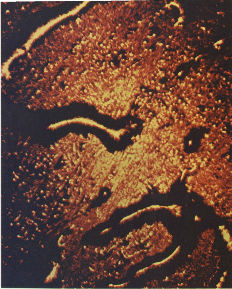
A dewetted surface was wetted initially but has pulled together upon solidifying to form the isolated globules.
