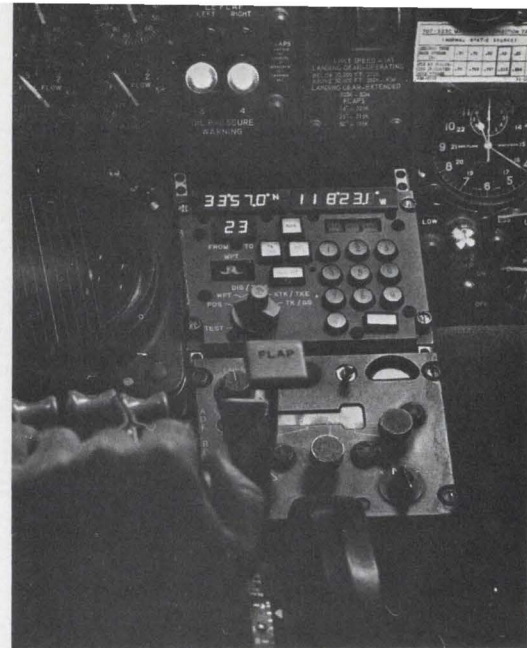
The Litton LTN-51 inertial-navigation units include, at left, the platform and computer system, a control display unit and a mode selector switch. On the right is the control display, as installed in the cockpit of an American Airlines plane during recent flight tests.
