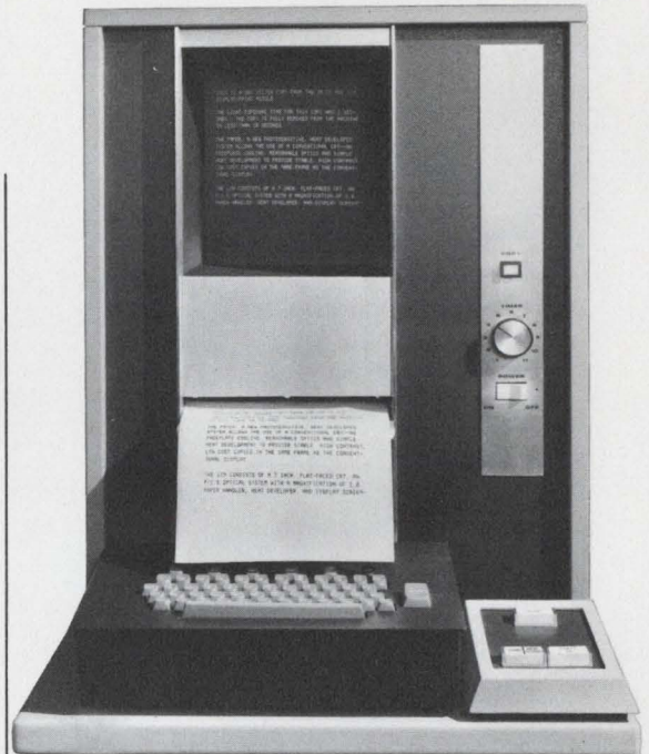
3M "129" Display CRT Print Module. Information retrieved from computer memory bank is displayed on screen at top. Press "print" button and information on screen will be reproduced on dry paper, below, within 10 seconds.
