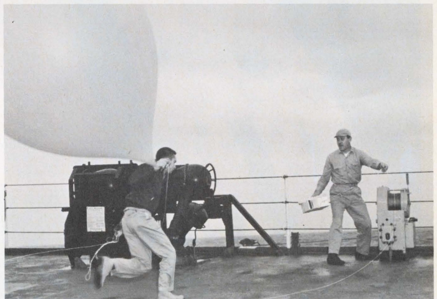
Weather balloons are launched every six hours from Coast Guard weather ships to provide meteorological data to the Weather Bureau and to commercial ships and aircraft. The SPQ-10 will track these to 100,000 feet and provide immediate outputs for teleprinter transmission.
