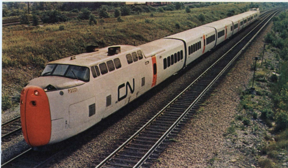
TurboTrains developed by United Aircraft's Sikorsky Div., will soon enter service between Boston and New York. Top speed will be about 120 mph.
