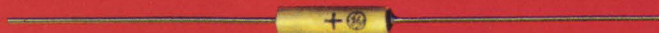
Tantalum Sub-miniature Wet-slug Capacitors 59 standard ratings. 6 to 60 volts, 0.01 to 450 \mu\text{f} , -40 to 85C ambient temperature
