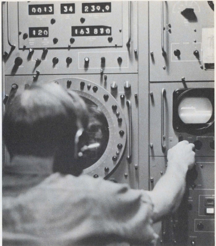
Combat Information Center displays are driven by the Honeywell DDP-516 general-purpose computer. Target data appear in the Nixie-tube displays (above), in the 12-inch scope (plan position indicator and range-height indicator), and in the range gate (right).
