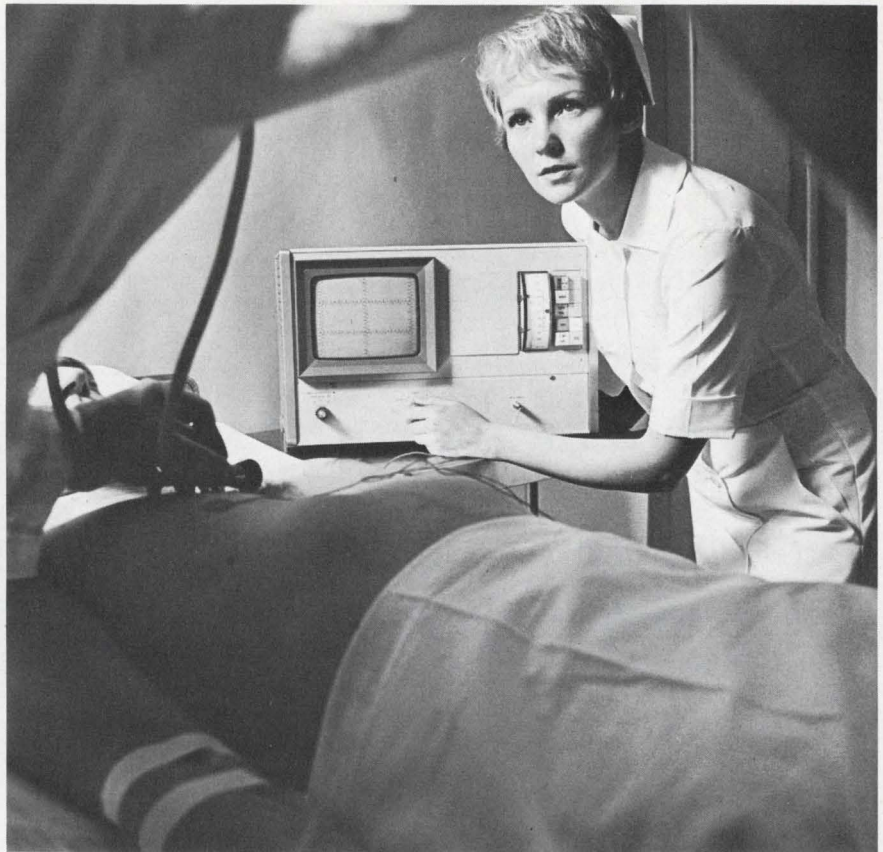
Bedside unit of patient-monitoring system contains an electrocardiogram channel, an oscilloscope display, a cardi tachometer, and an audio alarm. The unit was built by Honeywell, Inc., Denver.
