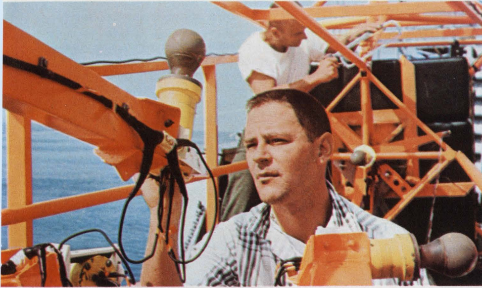
Hydrophones receive visual inspection before being lowered to the ocean floor from AC Electronics-Defense Research Laboratories' research vessel Swan.
