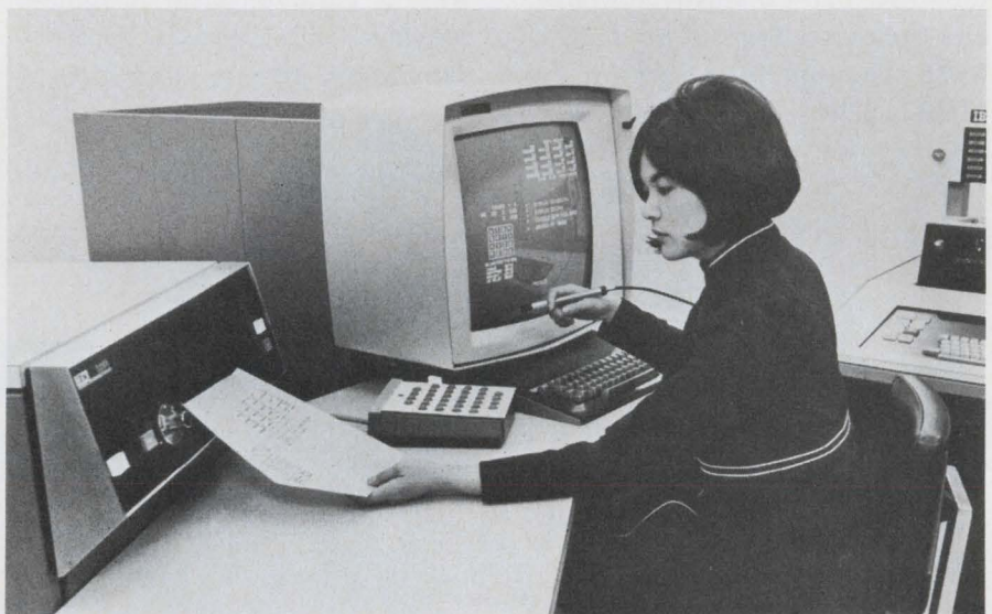
3. Copies from a graphics terminal can be made in 15 to 38 seconds in this system that uses IBM's 2250 unit and a new 3M photosensitive paper copier.
