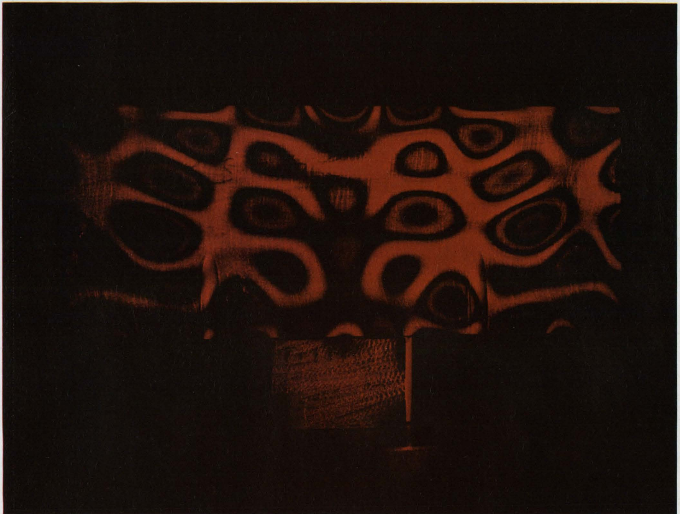
3. Holographic fringe patterns of deflection modes on the face of a 10 kHz sonar transducer element that was excited at 88 kHz. Made by the time-averaging method at the GE Electronics Laboratory, the bright areas are
