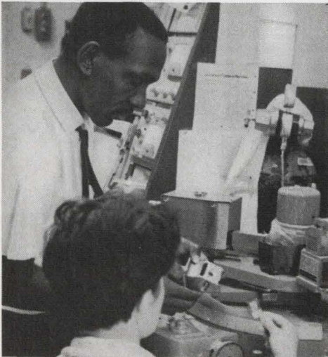
A Xerox scientist employs X-ray fluorescence in studying photoreceptors for current and future product use.
