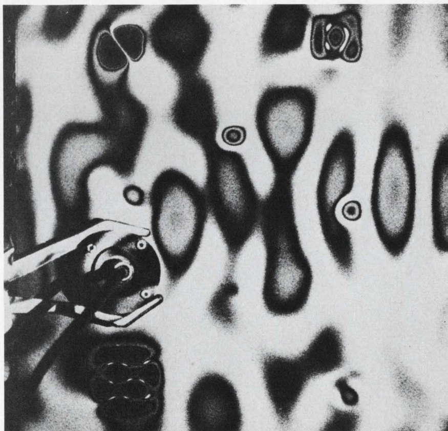
5. Clear indications of subsurface bonding flaws and voids in honeycomb panels can be seen by these fringe-pattern anomalies. At Aerojet General, the aluminum honeycomb surface was vibrated by the round transducer (in clamps). Flaws appear at 11,700 Hz, and stand out in marked contrast at 17,200 Hz.
