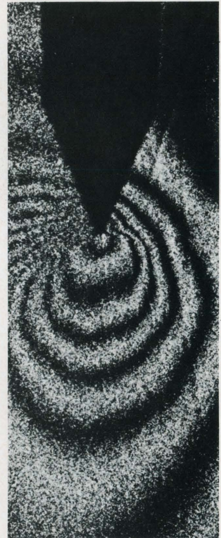
7. Holographic tests of metal toughness conducted by T. D. Dudderar of Bell Telephone Laboratories, show 12 microinch strain contours.
