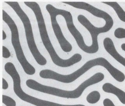
Before the bubbles are formed the magnetic domains look like fingerprint ridges and valleys. Domains shrink and bubbles appear (right). Bubbles shown above are about 1.4 mils in diameter.
