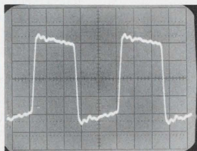
Fig. 17 Freq. 100 MHz Scope: 2 ns/div. 1 V/div.
