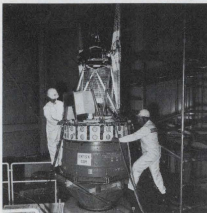
The ERTS will sense the earth's resources with three TV cameras and a multispectral scanner.
