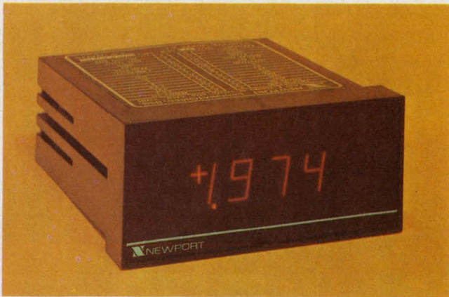
In Newport's Model 257, full-scale range and function are selected by means of a 16-pin DIP plug-in module. Full scale can go down to 19.99 mV.
