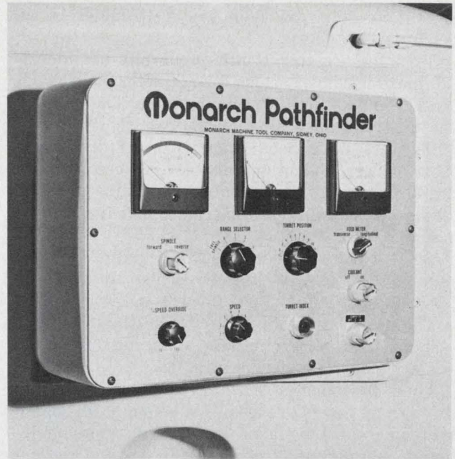
In a machine-tool application, Simpson's Model 1327—a 3-1/2-in. Wide-Vue meter—displays spindle rpm, motor load and tool feed in inches per minute.
