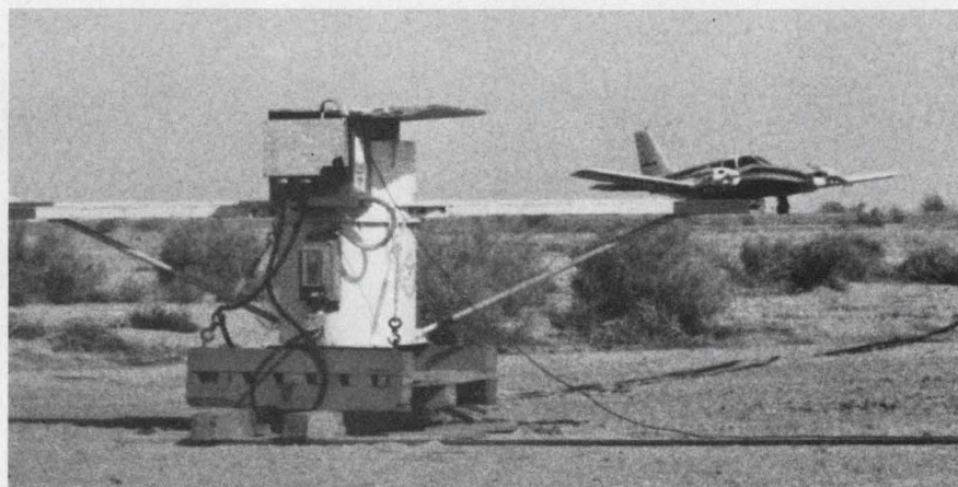
Experimental nuclear landing system beacon used for feasibility tests. The twin-engine aircraft (Piper Seneca) was used for flight system evaluation.
