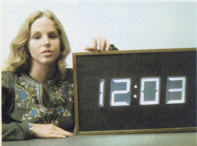
Large dynamic-scattering liquid-crystal displays that vary in height from 4 to 8 in. are available from Transparent Conductors Inc.
