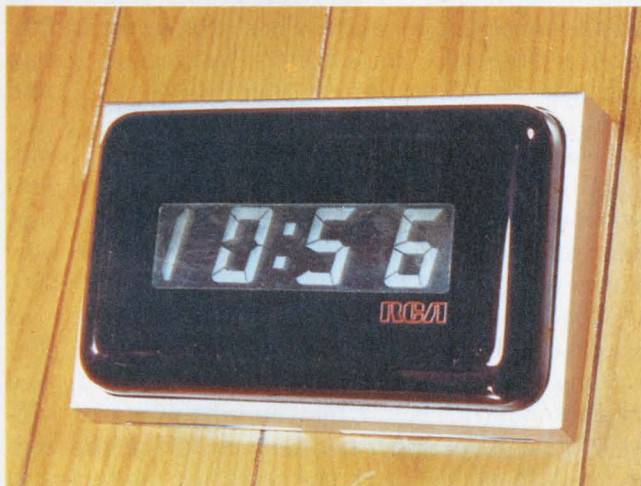
An experimental 2-in.-high, 3-1/2 digit dynamic scattering liquid-crystal readout, designed for digital-clock applications, has been fabricated by RCA.
