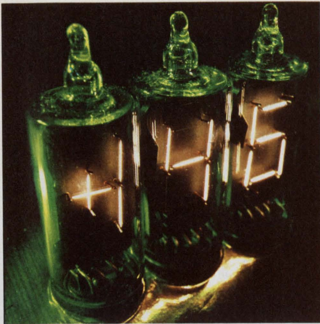
Incandescent displays that use directly viewed filaments, such as RCA's Numitron, can be filtered to produce a wide variety of colors.
