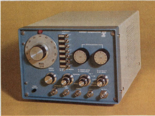
Internal switching in the Telonic 1210 couples two sweep sources and delivers a continuous band of frequencies from 200 kHz to 1000 MHz.
