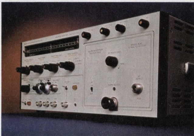
Single, dual or multiband plug-ins can fill the hole in Wiltron's 610C solid-state mainframe, a 100-kHz to 22-GHz box. Optional harmonic markers are provided in the video output, rather than the rf output.
