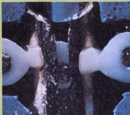
Cross section of TULIP™ contact termination.
