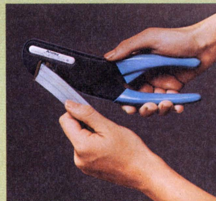
Pre-set compression cycle assures connection reliability.
