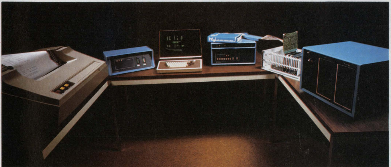
In-circuit emulation is offered in Intel's latest development system, the MDS. The capability permits early fault and error isolation in actual system prototypes.
