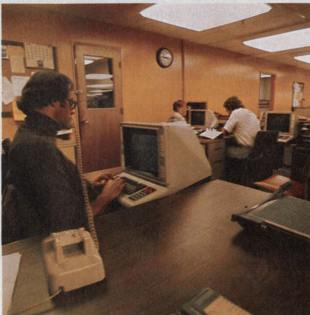
The 2644A Data Terminal from Hewlett-Packard uses a tiny version of the 3M data cartridge. On one track the cartridge can record over 100,000 bytes.
