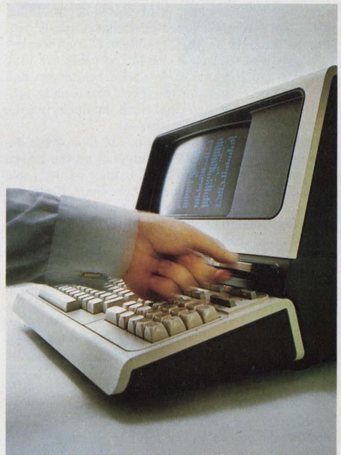
The 2644A Data Terminal from Hewlett-Packard is a smart terminal with a character generator that can draw line segments and a pair of built-in data cartridge drives that accept a new, small 3M data cartridge. The cartridges can be used on-line as well as off-line.
