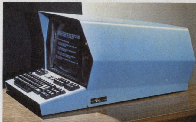
The Model 455 from TEC, Inc., is a smart terminal with a large character set and a full range of editing functions and cursor controls.
