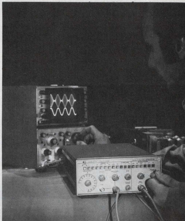
AM or FM control, along with sine, square and triangle waves, is available on the 3312A, a $900 13-MHz function generator made by Hewlett-Packard.
