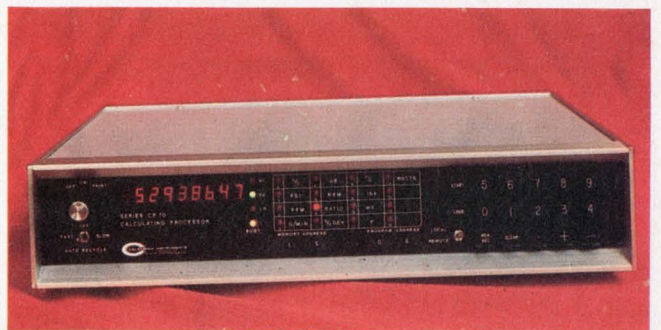
A calculating processor, the CP 70 from California Instruments, depends upon an internal LSI chip set. The unit performs calculations upon data received from a variety of instruments. The processed results are shown on an eight-digit LED display.
