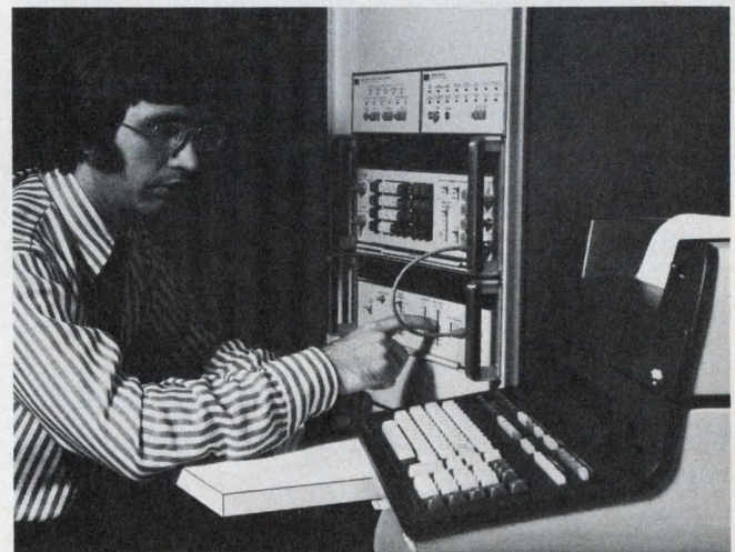
The frequencies to which the synthesizer of the HP 3045A Spectrum Analyzer are stepped is controlled by the calculator. The spectrum bandwidth is also under program control.
