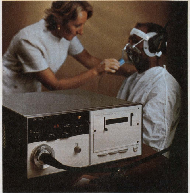
Blood oxygen can now be rapidly monitored with this HP 47201A noninvasive oximeter. Readings are taken 20 times per second.
