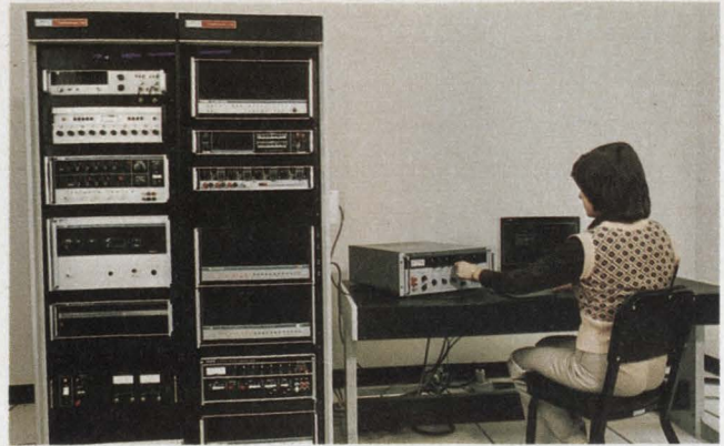
Calibration of dc and ac calibrators, DMMs and analog and differential voltmeters is performed by the Fluke Terminal/10, a computer-automated precision tester.
