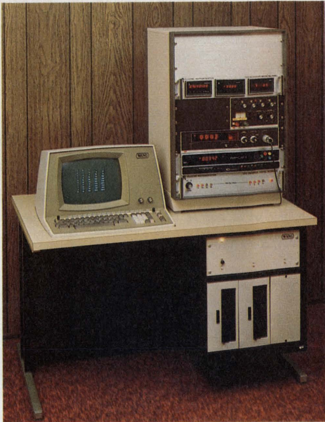
Automatic measurement and storage of resistance values for telephone-connector contacts is made with this Fluidyne system. A Wang WCS/20 calculator with a disc file is used.
