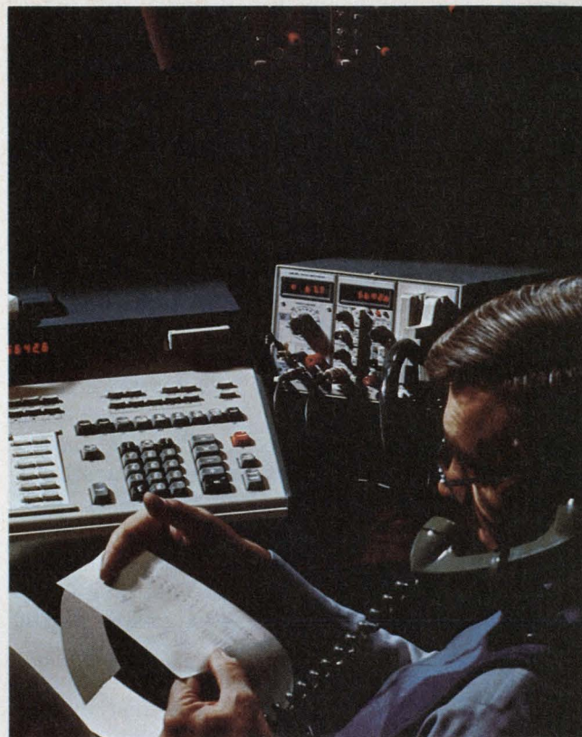
A magnetic tape cartridge in the Tektronix 31/53 calculator provides automatic data acquisition, logging and statistical routines for interchangeable plug-in modules.
