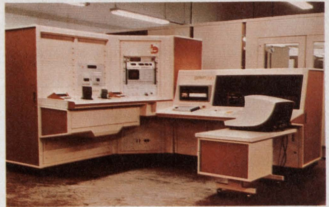
For circuit boards containing \mu Ps, the System 390, from Instrumentation Engineering, offers a word generator/receiver that produces large pattern arrays.
