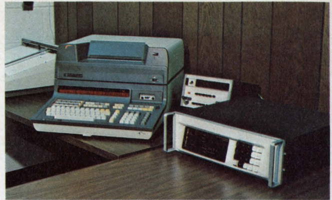
Testing and calibration of PC circuit boards is provided by the Wavetek 159 programmable function generator shown here, under the control of an HP 9830 calculator. The Wavetek instrument is designed with an HP-IB compatible interface.
