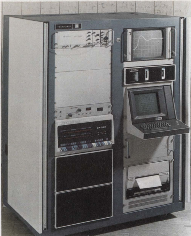
Digital waveform analysis of transients with up to 500-MHz bandwidth is recorded and displayed by this Tektronix Waveform Digitizing Instrument.
