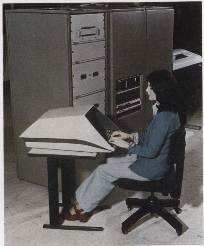
Hot off the assembly line is the Siemens/Computest 203, a semiconductor memory test system that runs various tests at a blazing 20-MHz rate.
