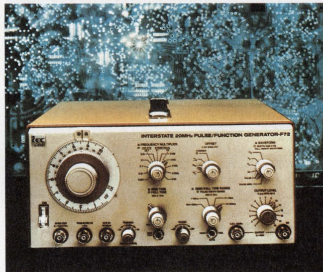
The 20-MHz Model F-72 pulse/function generator made by Interstate Electronics offers the user variable pulse rise and fall times and sine, square and triangle output signals with variable offsets.
