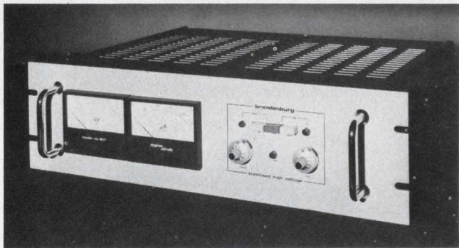
Up to 30 kV at 500 \mu A is available from Brandenburg's Model 827 high-voltage supply. The unit can be adjusted over 0 to 30 kV and has dual meters to monitor the output.
