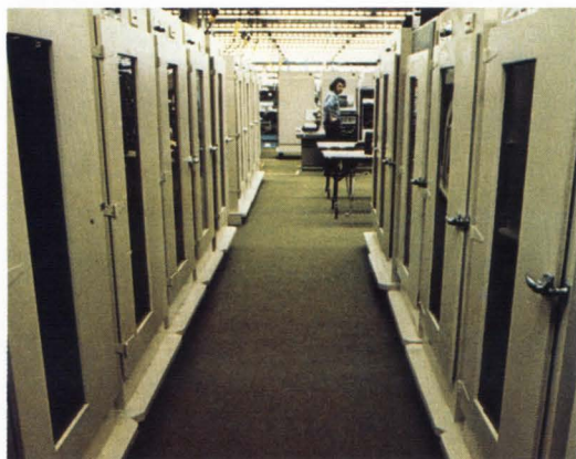
Temperature chambers stress computers to isolate marginal components. Computers are continuously tested during 72-hour burn-in at 50°C. Any error starts the test over from the beginning. To further stress the computer, power is cycled on and off approximately 2000 times during test.
