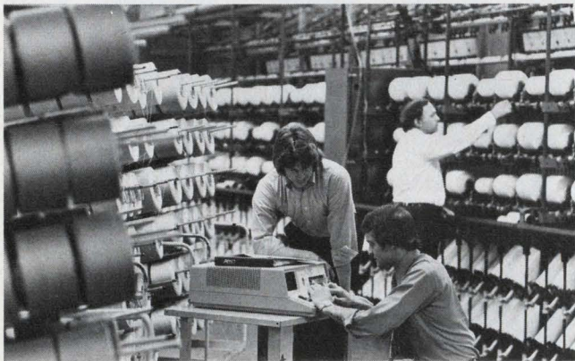
A computer model of a textile mill that runs on an IBM 5100 computer is used to examine production rates and calculate manufacturing costs.
