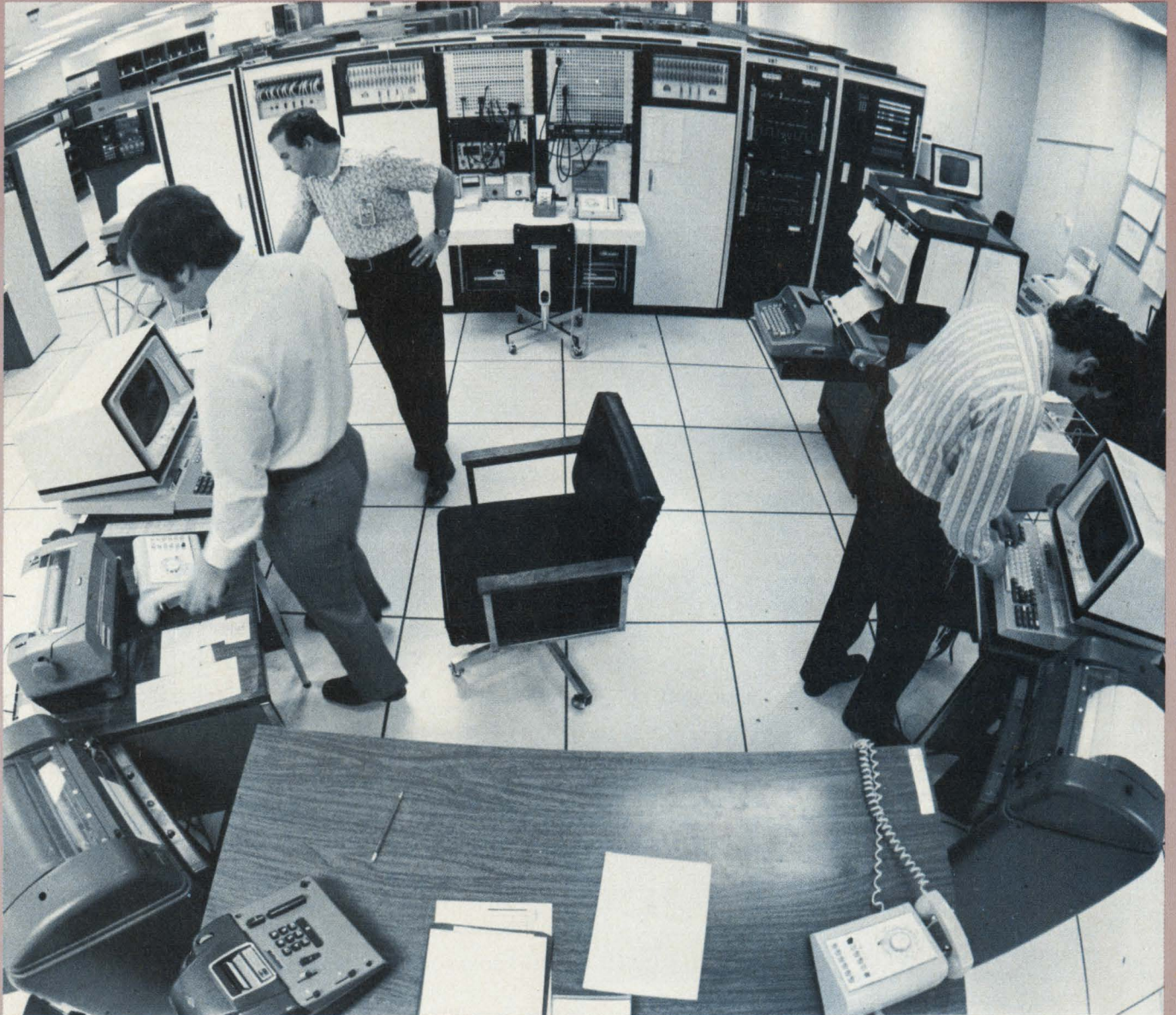
Trans World Airlines computer reservation system runs on an IBM System/370 Model 168.
