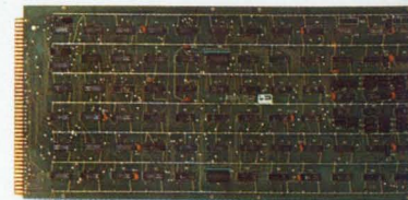
16-channel Priority Interrupt Module. Model 13220-00. 16 interrupts with acknowledgement lines.
