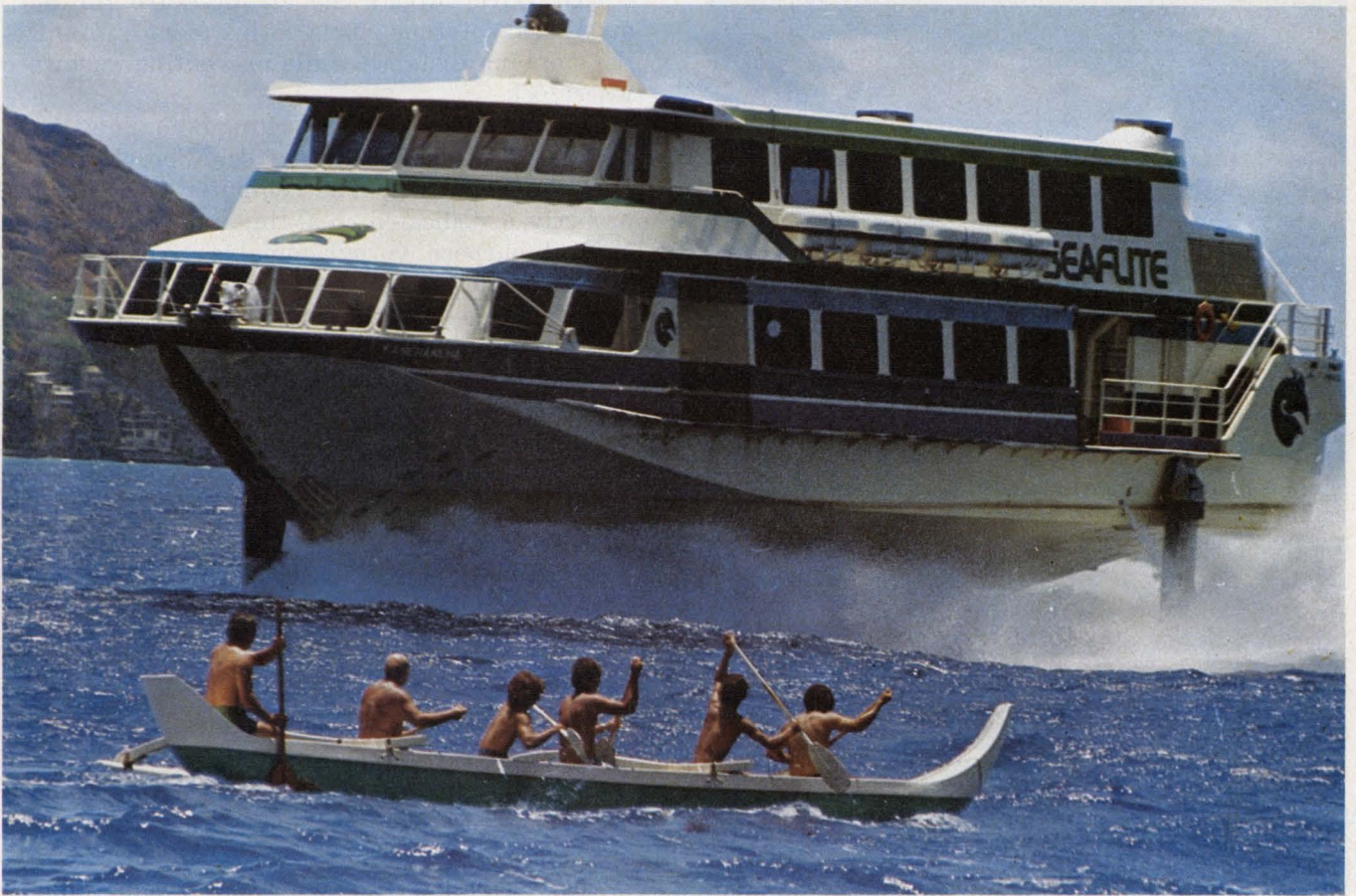
An analog computer ensures the smooth ride of Boeing's surface-skimming hydrofoil. On board, an automatic control system stabilizes the craft and controls trim and altitude while compensating for disturbances in the sea.
