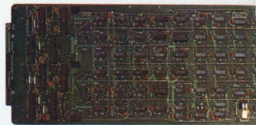
I/O Distributor. Model 14629-XX. In conjunction with Intelligent Cabling (see text), the I/O Distributor provides up to eight interfaces—serial or parallel in any mix. Small version accommodates four interfaces. A DMA version allows data transfer rates up to 250K bytes per second.
