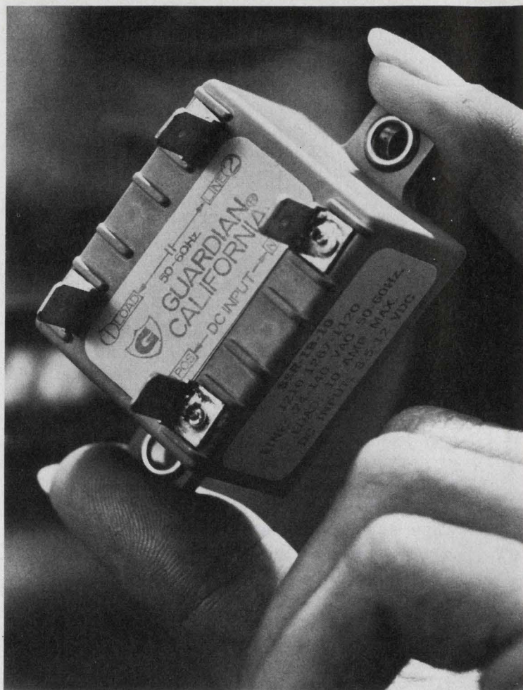
A nylon case covers the innards of this SSR. The relay is mounted on an isolated metal base to provide good heat conduction to an external heat sink. Guardian Electric rates these units for loads of 7 to 10 A and up to 280 V rms.
