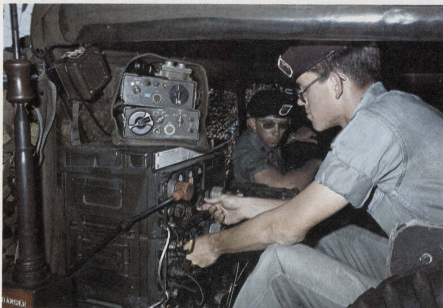
The 82nd Airborne Div.'s AN/VSC-2 radio-teletypewriter terminal is air-droppable, lightweight and long-range. Mounted in a jeep, it uses an AN/GRC-106 single-channel, hf, SSB radio with a frequency-shift modem.
