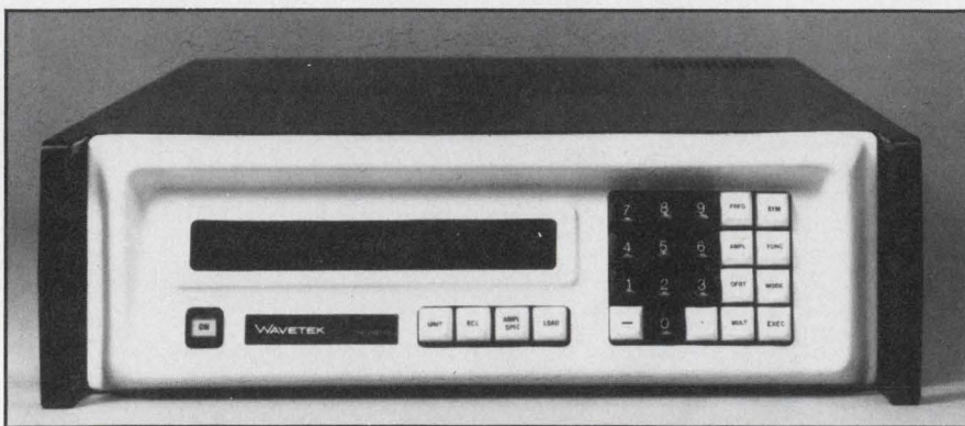
3. Instruments that talk back, like this Wavetek 172 Waveform Source, would not be practical without \mu Ps. Neither would the complex 172's front panel.
