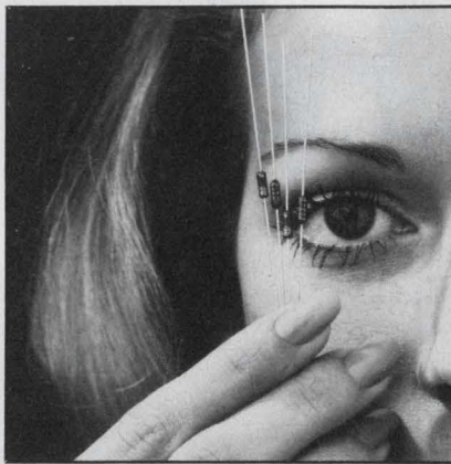
A new "universal" film resistor, the type-cc cermet from Allen-Bradley, has standard 1% and 0.5% tolerances and dissipates 1/2 W.
