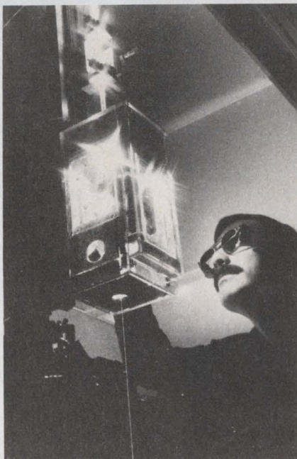
Glass rod is heated in an oxyhydrogen torch to remove surface flaws and air bubbles.
