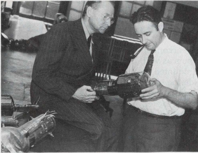
An experimental electronic-imaging tube examined by Zworykin, seated, and Dr. George A. Morton of the RCA research staff in Camden, N.J. during the late 1930s.
