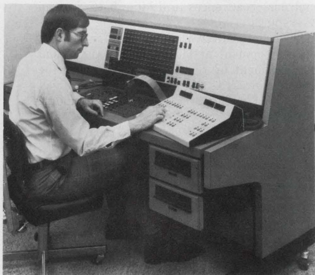
Four processors running in parallel allow the user of the Fluke Trender 3040A to test microprocessors at clock rates up to 10 MHz. Stored sequences run at 1.5 MHz, and automatic sequences operate at 5-million patterns per second.
