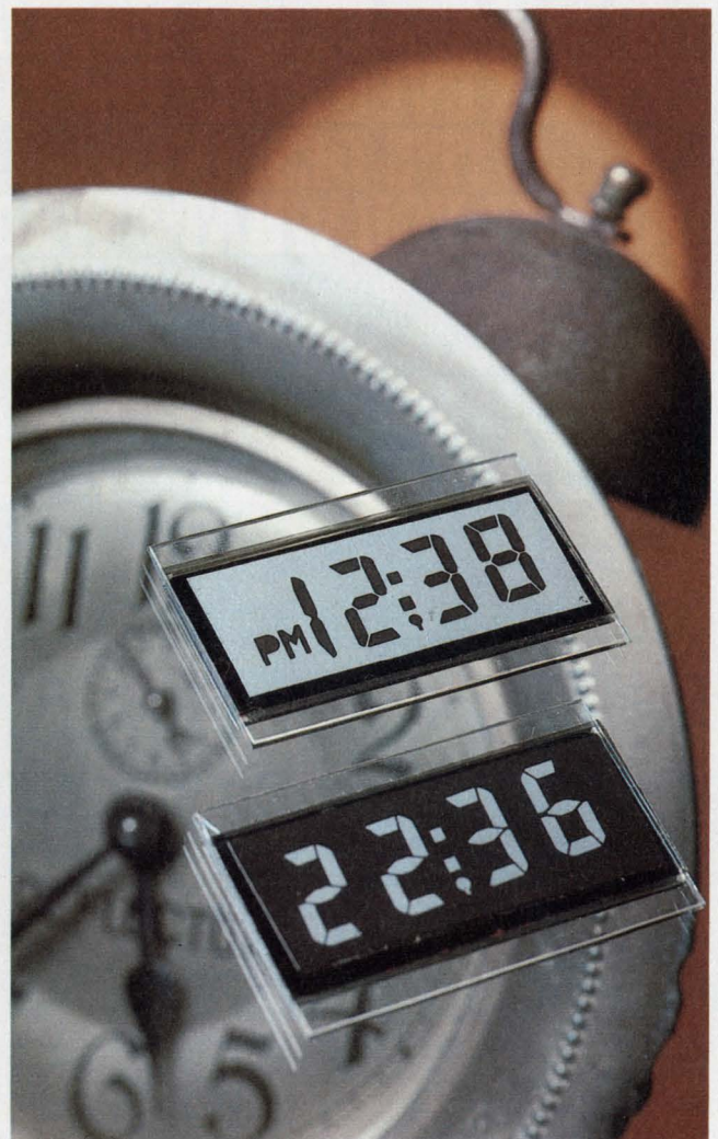
Liquid-crystals use the lowest power of all displays. This clock display by Hamlin draws only a few microwatts with all digits energized.
