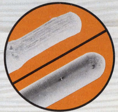
The dramatic difference in wear between Bonded Lubrication and ordinary contacts is shown by these electron images.
