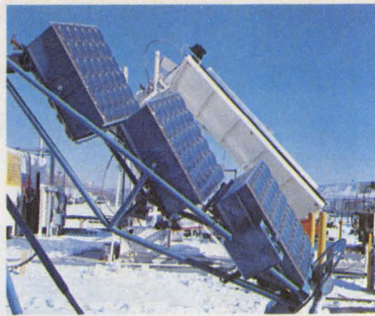
This two-axis, three-section tracking concentrator generates 300 W p , and uses a solar-powered \mu P and stepping motors to follow the sun. RCA expects this "fly's eye" concentrator to cost $1/W p in volume quantities.
