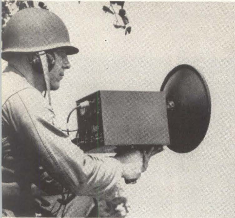
Army also wants smaller radar, like this experimental 10-lb set
