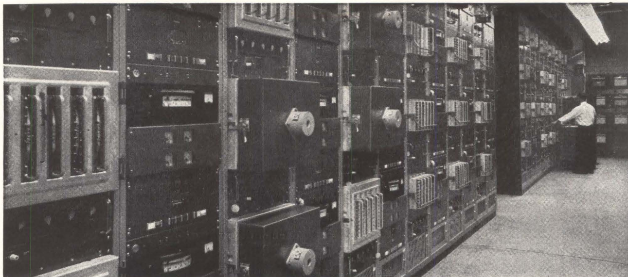
Banks of racks are used for d-c dissipation tests of transistors. Small detachable ovens with individual temperature control can be placed over selected racks for testing at elevated temperatures. Special techniques are used to prevent the testing operation from introducing failure from wrong connections, overloads or voltage transients
