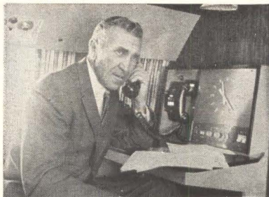
Typical private aircraft installation. The second phone is the aircraft intercom. At right is airborne telephone package manufactured by Delco as the CAT-2 Skyphone
